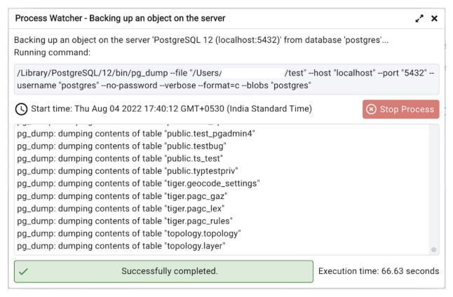
The Process Watcher logs all the activity associated with the process/task and provides additional information for troubleshooting Use the **Stop Process** button to stop the Backup process.
